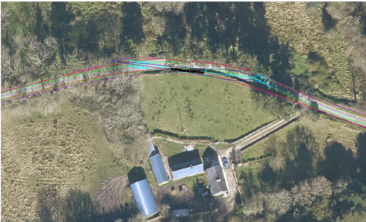
Figure 47 - Pinch point at Chainage 825m - swept path
