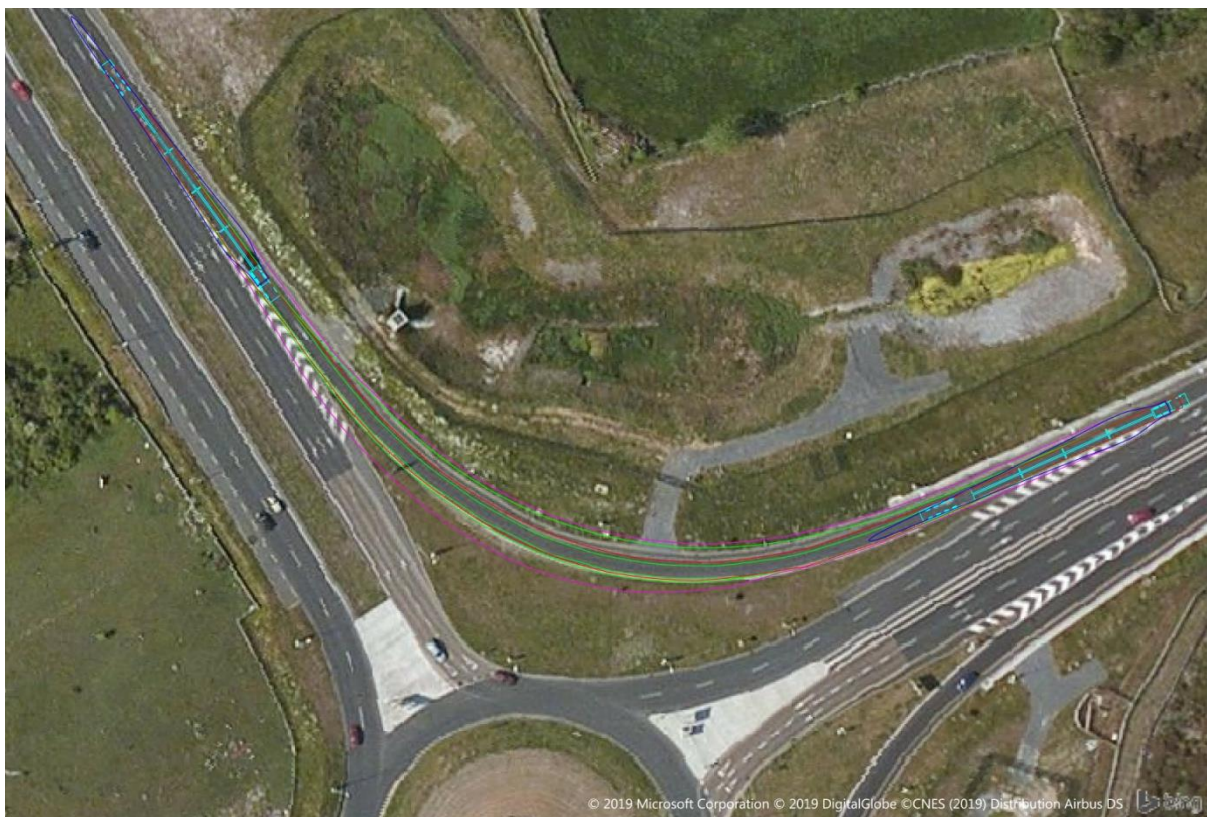
Figure 14 - Exit from Bothar na dTreabh (N6) to M6 eastbound - swept path
