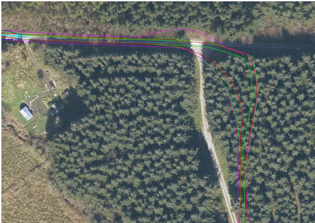
Figure 50 - Proposed modifications to existing entrance - swept path
