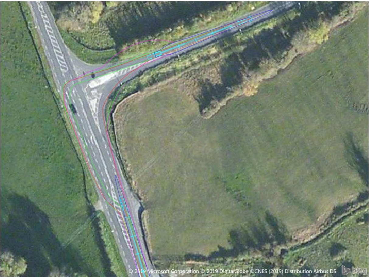
Figure 25 - Junction of Foynes Port road with the N69 - swept path
