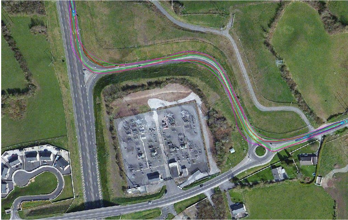
Figure 20 - Junction 13 south bound - swept path
