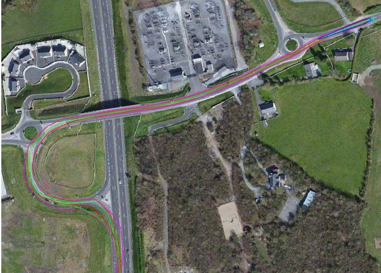
Figure 34 - Junction 13 north bound - swept path
