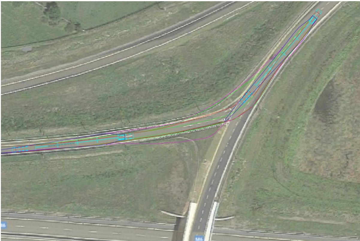
Figure 17 - Swept path for entry to M6 / M18 interchange - swept path
