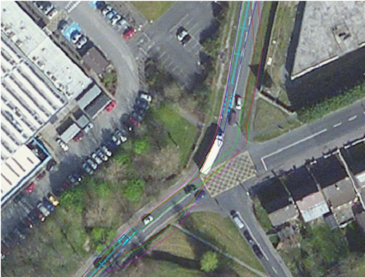
Figure 10 - Left turn from the R339 towards Tuam Road - swept path
