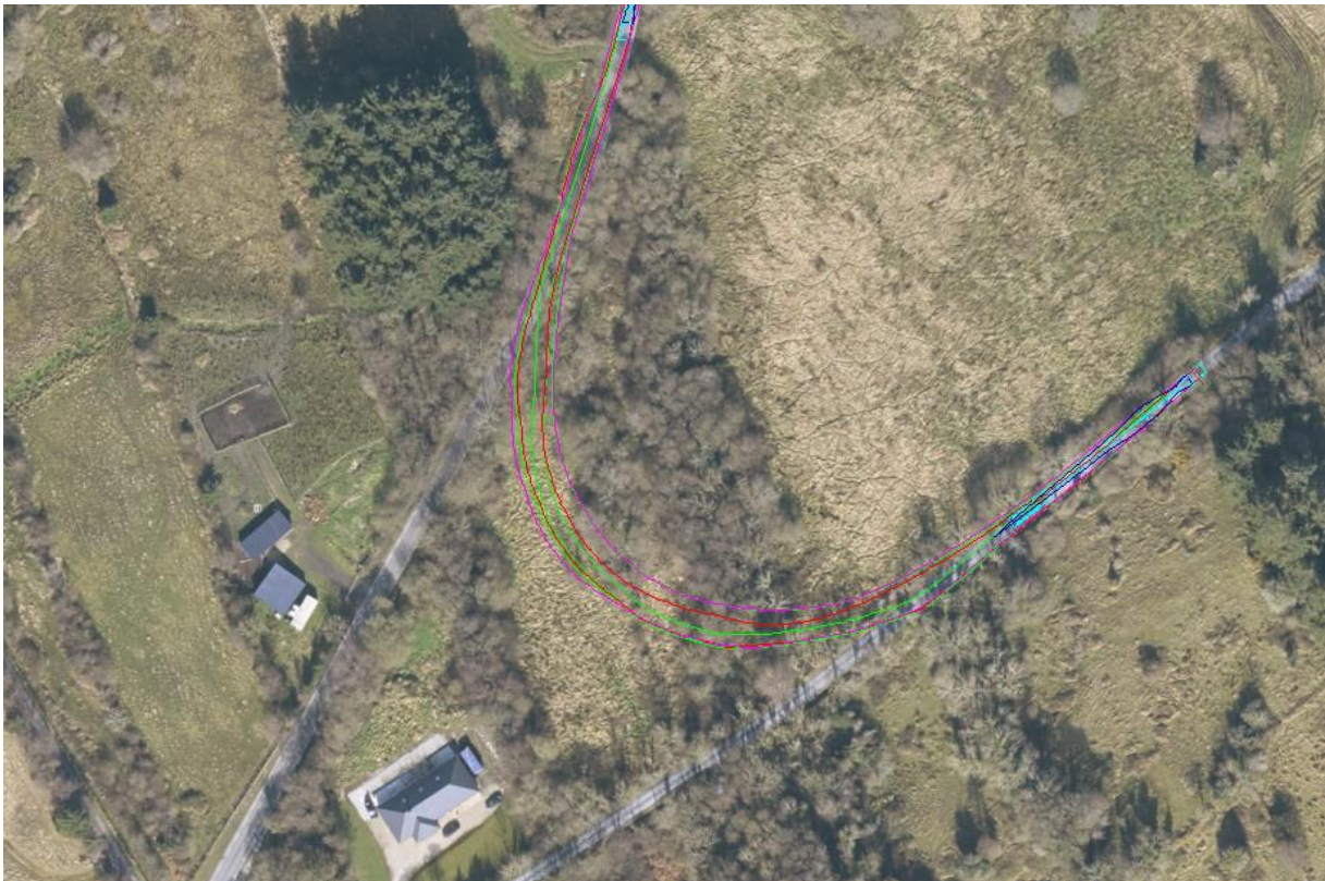
Figure 43 - Bypass route from R465 to the local road - swept path
