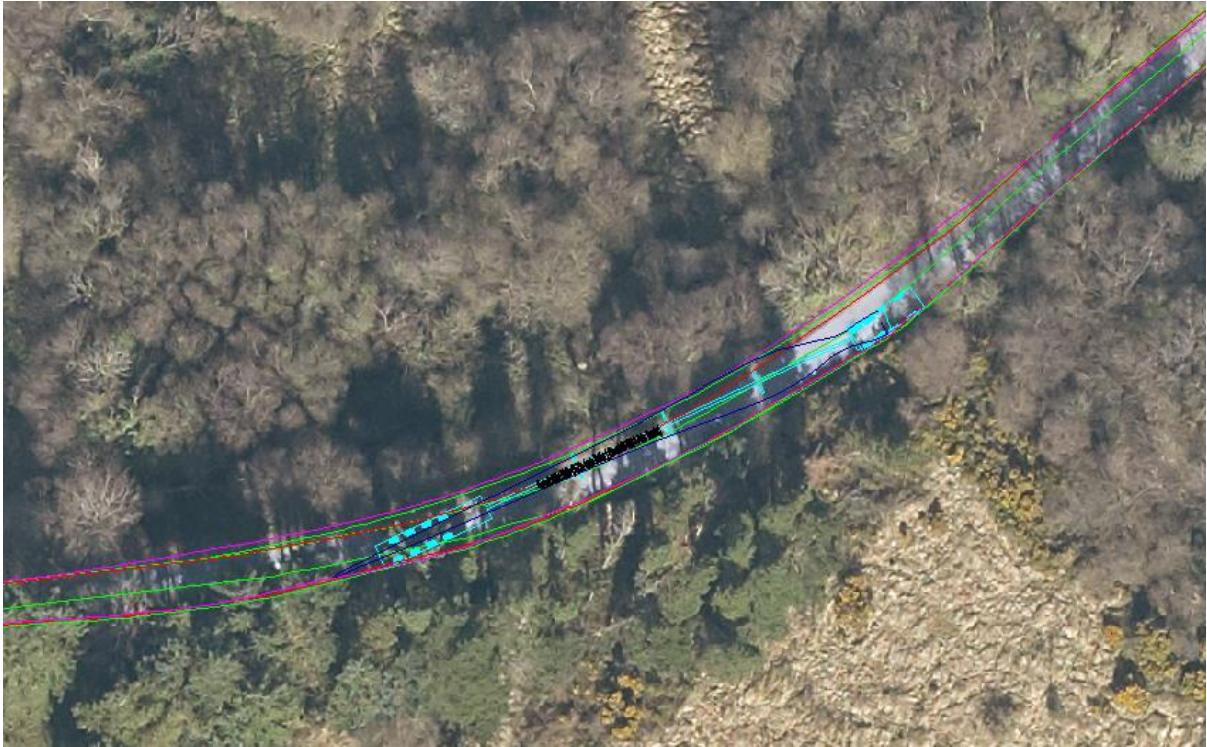
Figure 46 - Pinch point at Chainage 490m - swept path
